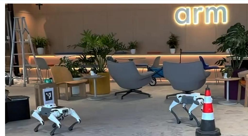
MAPPO navigation with obstacle avoidance on real robots. Robot Demo credit: Waheed Brown, Arm
